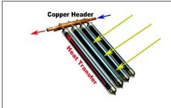
The heat pipe is a very efficient means of transferring heat from within the evacuated tube to the water. The following diagram shows both the glass evacuated tubes and the copper heat pipe. The heat pipe is simply inserted into the glass tube, held in place with high quality silicon based cap.
