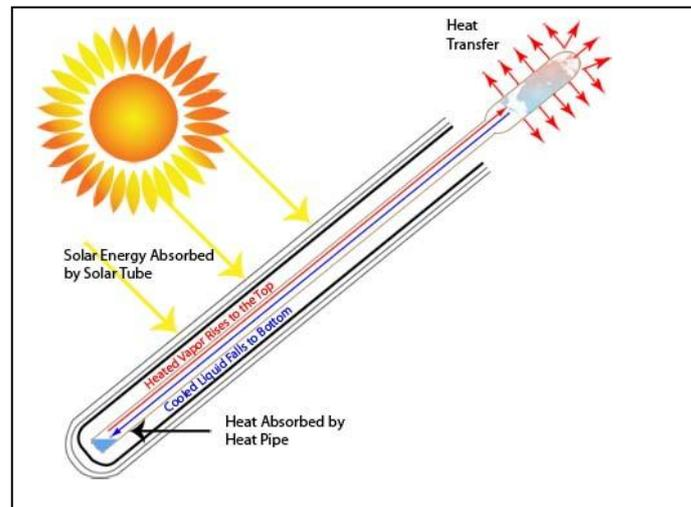
This method of heat transfer is thousands of times more efficient than a solid copper rod. Heat is therefore very efficiently transferred from the glass evacuated tube to the water. Since no water is flowing through the collector tubes and the tubes are hermetically sealed it does not suffer from corrosion problems as is the case with other solar collector types.
