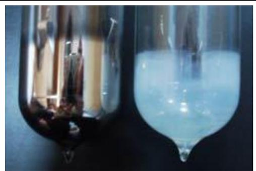
The Getter is located at the bottom of the outer tube.
